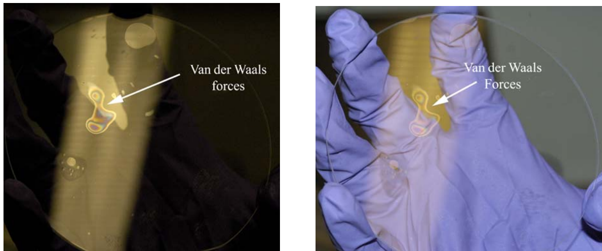
Figure 1: Van der Waals forces shown in fused glass substrates (left and right picture) that were pressed together without vacuum.
